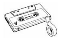
**Note:** When covering the holes, cover only the place that was originally protected by the plastic tab.
